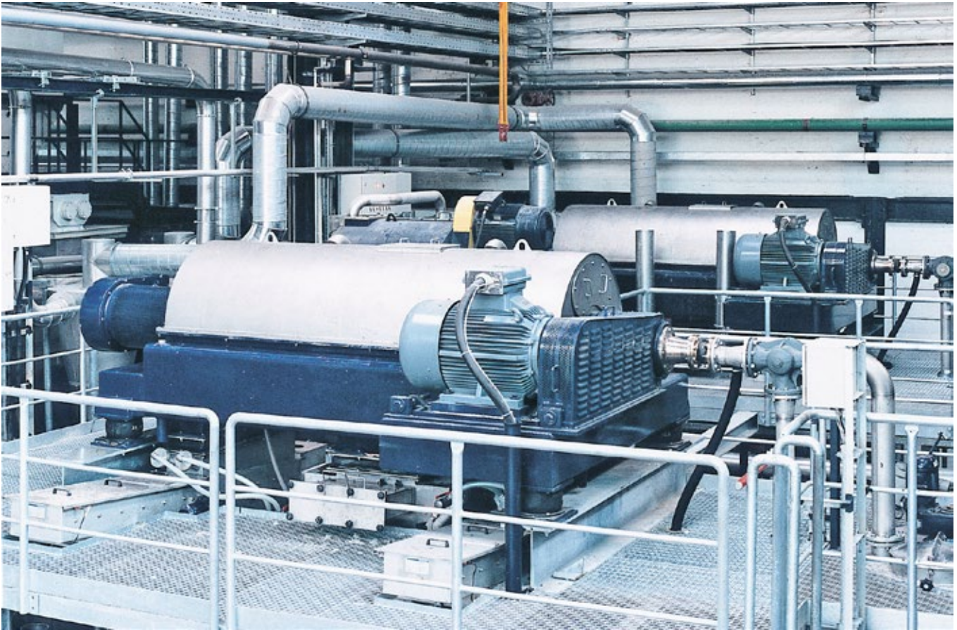
Two-stage ANDRITZ decanter centrifuge ACZ installation for sorting mixed plastics and producing absolutely pure PA granulate.
