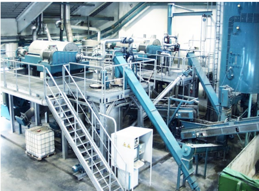
Two-stage ANDRITZ decanter centrifuge ACZ installation for sorting mixed plastics and producing absolutely pure PA granulate.
