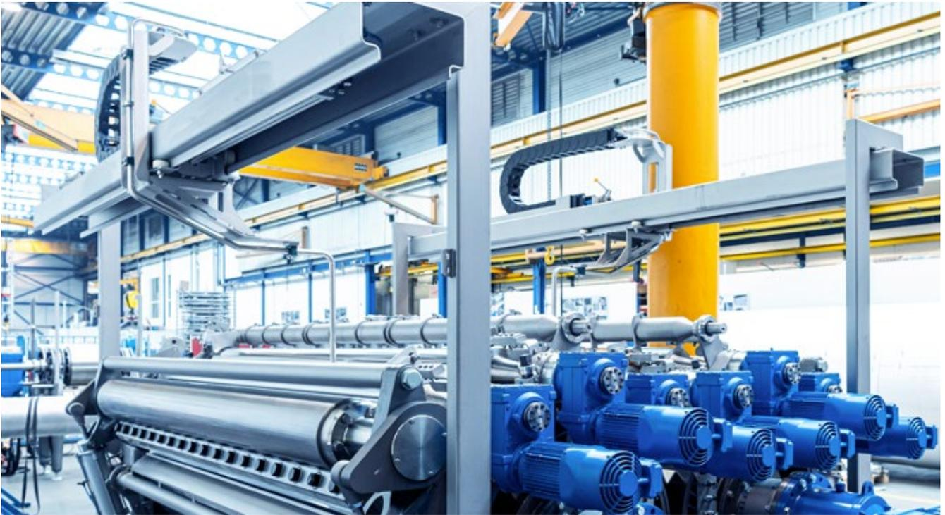
Drum dryer with linear feed system
