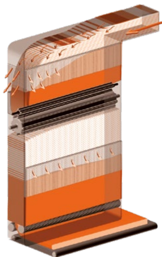
TCF-X: Self-regulating fiber distribution system in cross direction
