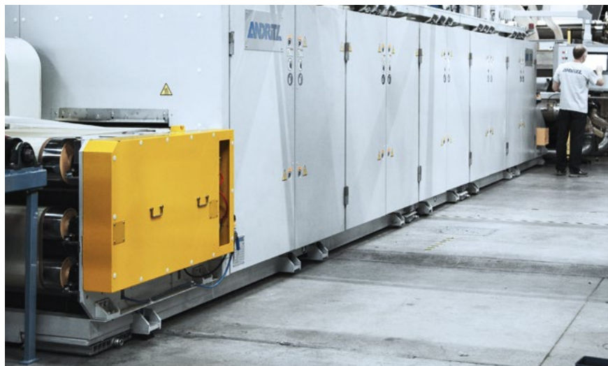
Flat oven of the ANDRITZ air-through-bonding line at the CETI
